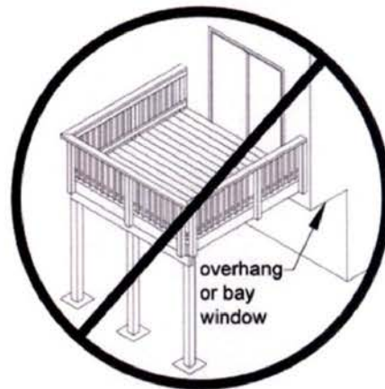
Figure 18. No Attachment to House Overhang with Ledger.
